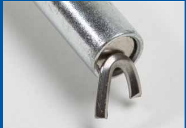
The magnetic tang-break tool at work
